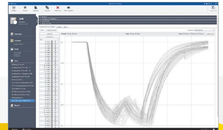
Easy management of location, asset and test data due to a structured database, implemented search and filter functions and automatic data synchronization.
